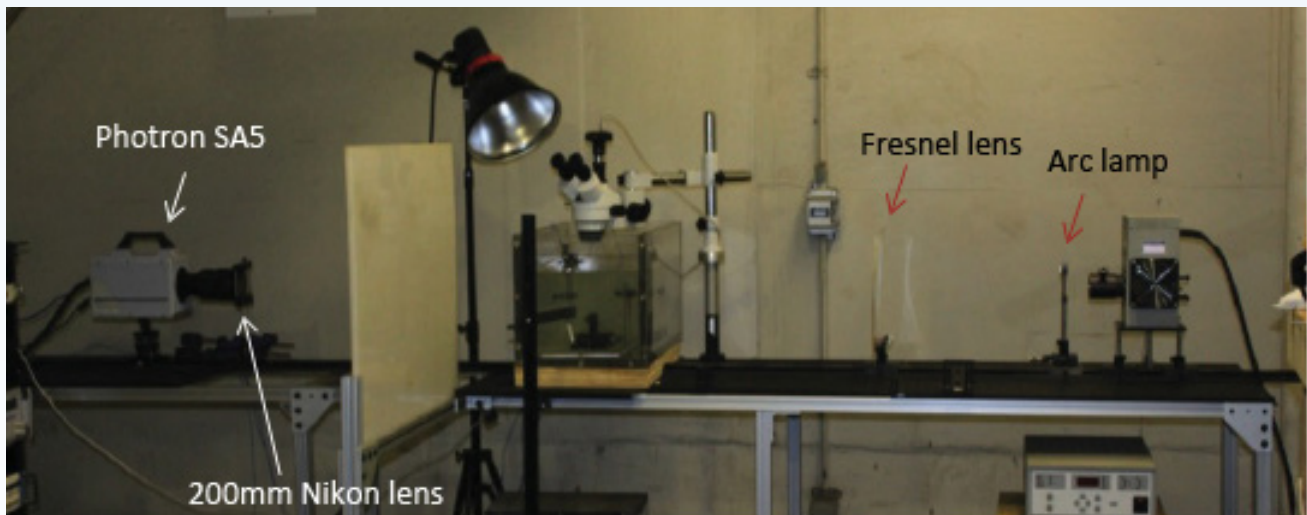
Figure 8-1: A Modified Aquarium Setup for Performing Blast Experiments Underwater
