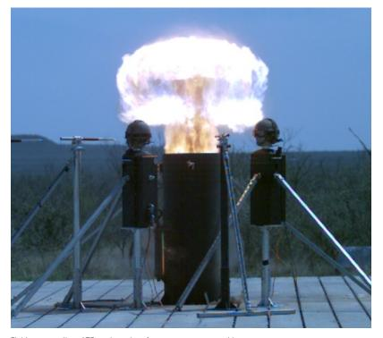
Field test to collect ATF eardrum data for exposure to mortar blast
