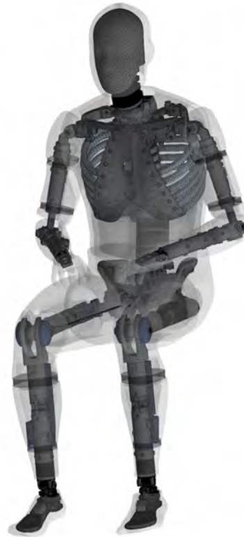
FIGURE 6-9: Response of the WIAMan ATD When Used Within a Simulation of a UBB Attack on a Full Vehicle (Photo courtesy RDECOM)
