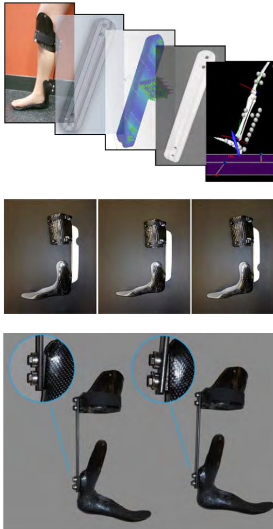
FIGURE 7-20: Top Image: 3D printing methods (selective laser sintering) modified the stiffness of the IDEO®'s posterior strut.
