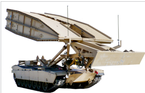
FIGURE 1: An AVLB launcher integrated onto a M1A1 Abrams Chassis (Figure used with permission of the authors)
