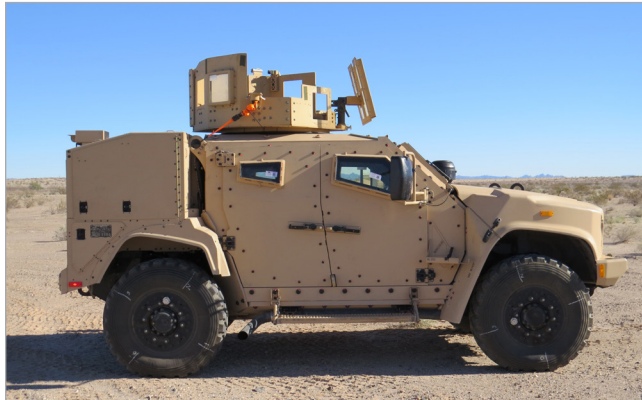
FIGURE 1: JLTV-Close Combat Weapons Carrier (CCWC) Variant (Figure used with permission from the authors)
