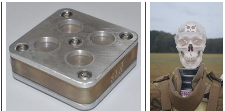
Figure 1. A) The cell pack is a 5 cm square device with four independent cell culture wells capable of supporting 3D neuronal cultures for up to 2 weeks. B) The cell pack in a gel-based brain (rear half) in a surrogate headform. Not shown are the front gel-brain half that fits tightly against the cell pack and the skull cap form the full head.
