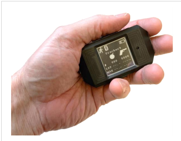
Figure 6. Blast Tracker 2 gauge including microphone and accelerometry
