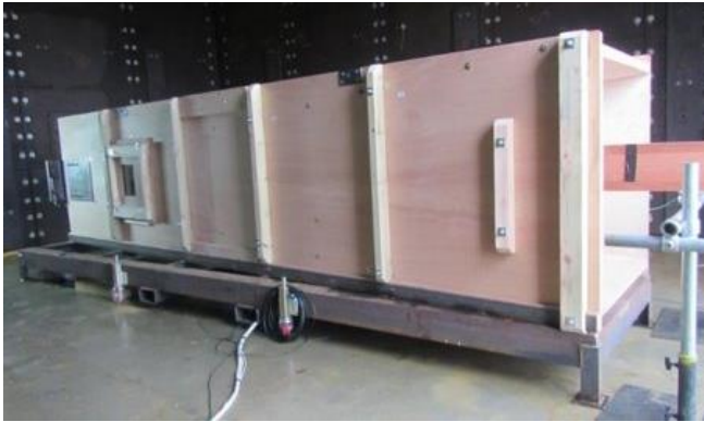
Figure 8. Design principle and prototype of a device that models exposure to blast waves.
