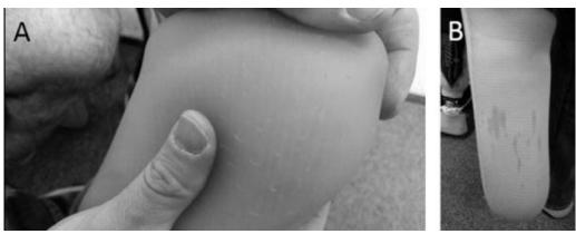
**FIGURE 3:** A, Interior of liner showing perforations. B, Exterior of fabric covered liner showing wet patches where sweat was absorbed during active wear. These sweat patches appeared after approximately 5 minutes of light jogging indoors in a patient that has reported sweating as a problem. (Figure 2 from Caldwell and Fatone (2017) used with permission from the authors)
